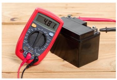
Fig. 1.1.5: Measurement of DC voltage
