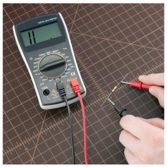
Fig. 1.1.7: Measurement of resistance
